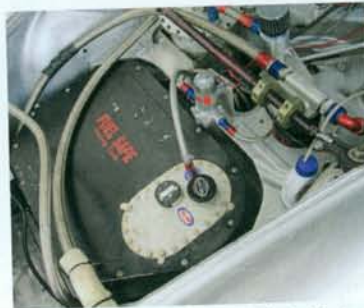
There are now so many different kinds of fuels and additives you can't say with any certainty how the fuel cell foam is going to interact with the fuel. You're simply going to have to monitor your own situation. If you think you have an issue you can talk to the fuel cell makers. They should be able to provide some guidance.
