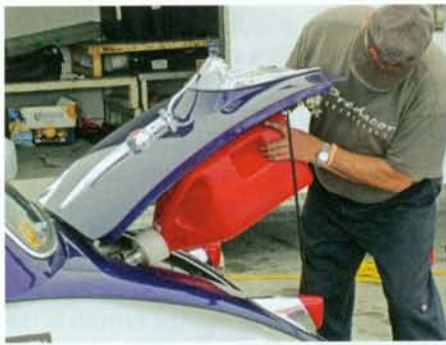
These red jugs are much better for storing gasoline than the clear jugs. Most (but not all) gasolines are photosensitive.
