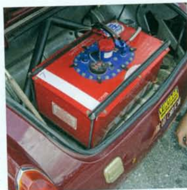
Given the nature of the new gasoline formulations you might be better off with a new fuel cell than your old gas tank because of varnish in the tank. A fuel cell is also far safer in a crash.
