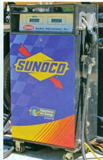
◀ Sunoco brings these portable pumps to the Indy car races. The gas is pumped directly from the tanker truck. Most of the major fuel suppliers seem to be moving away from using underground tanks.
