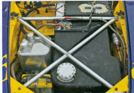
This Porsche 935 uses a combination of braided steel and braided fabric fuel lines. Some of the new race fuels may not be compatible with these older fuel lines. Call the fuel line manufacturer and ask questions.
