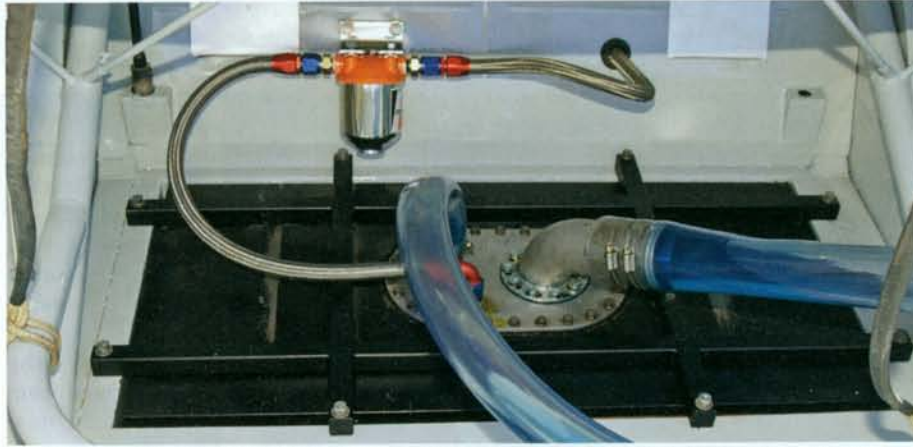
This is going to be an easy fuel filter to change. Change filters often—more often if the fuel has a blend of ethanol.
